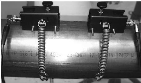
FIGURE 40: V-mode or W-mode with spacer bar
