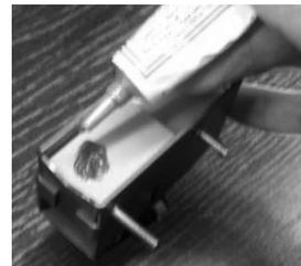
Apply acoustic gel on the sensing face of the ultrasonic transducer.
