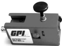
Ultrasonic transducer QMP-F21 (2 MHz), RED housing, for pipe diameters from 0.5 to 4.0 inches. Operating temperatures: -40° F to 300° F
