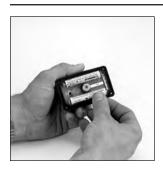
When the batteries are installed correctly, the computer powers on automatically. Check the readout to make sure normal meter functions have resumed before assembling again.
