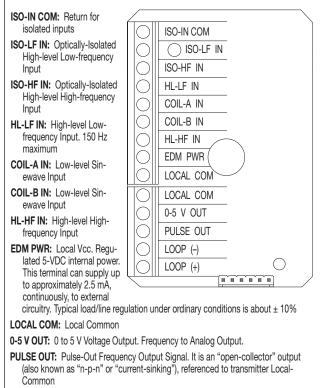
LOOP (-): 4 to 20 mA Current Loop - current into transmitter
