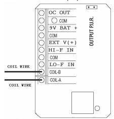
Connect either coil wire to COIL\_A terminal.
