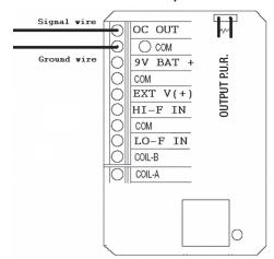
Connect signal wire to **OC\_OUT** terminal. Connect ground wire to **COM** terminal.
