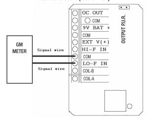
Connect either wire to **LO-F\_IN** terminal. Connect other wire to any **COM** terminal.
