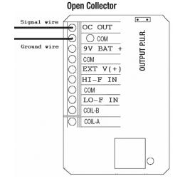
Connect signal wire to **OC\_OUT** terminal.
