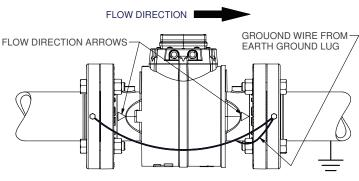
TYPICAL INSTALLATION IN STEEL CONDUCTIVE PIPE TO MAINTAIN GROUND CONTINUITY (ANSI Flange Version Shown)
