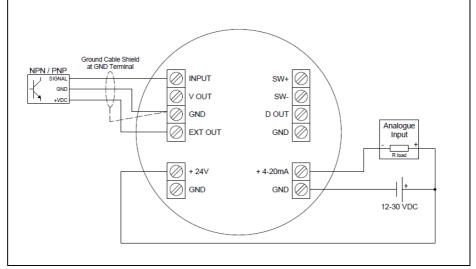
Note: Some instrumentation systems may have a common ground between the analogue input and the DC supply, for those systems this wiring configuration will not be possible and configuration 4.3.8 must be used.
