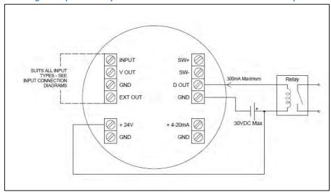
Note: Wiring connection from voltage supply to +24V terminal on instrument is not compulsory, however it will prolong battery life.
