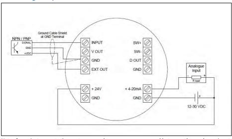
Note: Some instrumentation systems may have a common ground between the analogue input and the DC supply, for those systems this wiring configuration will not be possible and configuration 4.3.8 must be used.
