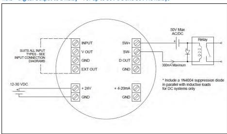
Note: This output type is not internally protected from voltage spikes from inductive loads, a diode must be fitted as shown for DC loads, or a Metal Oxide Varistor fitted for AC circuits.
