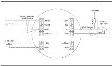
Notes: Shown here with Reed Switch input, Coil and Voltage Pulse inputs also suitable for this configuration. \*External 12-30V DC power supply to instrument is optional.
