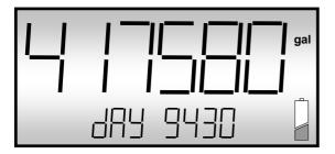
Full LCD display test feature illuminates all display segments and script text displays for 5 seconds when entering the program mode.
